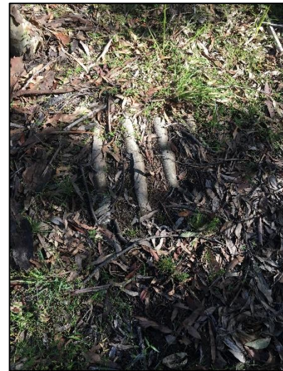
Plate 35: Corrugated ACM sheet partially buried in leaf litter to the north of sample location SS41.
